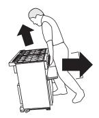
Lift the front of the cooker slightly and pull forward.
